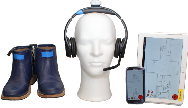
Fig. 4. Hardware for localization and 3D audio voice radio communication. The OpenShoe units (integrated in the sole of the shoes) and the stereo headset are connected to the Android platform (tablet for the commander and smart-phone for other agents), which rely on a WiFi network for communicating with the Android platforms of other agents. Cables are not displayed. The Ubisense radio tag provides synthetic inter-agent range measurements.
