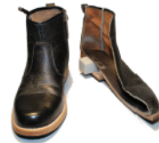
Fig. 1: Shoes with units of the presented foot-mounted INS implementation integrated in the heel and casing with USB connectors at the shoe shafts.
